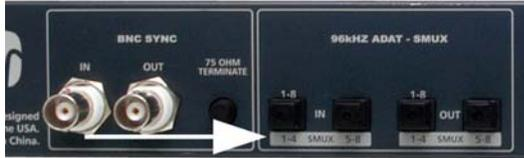
SMUX, a newer generation of optical light pipe technology, supports sample rates up to 96k and utilizes two optical cables for channels 1-4 and 5-8, respectively.
