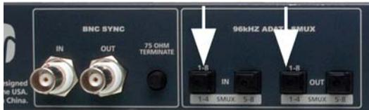
ADAT is an optical format that supports eight channels of digital audio over optical light pipe. Supported sample rates are 44.1 and 48k.
