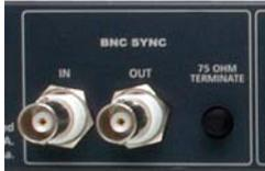
Many engineers prefer to take care of word clock and audio separately from each other, and you will find BNC cables used to deliver word clock in many quality studios and broadcast facilities worldwide. BNC cables are more rugged, lock into position, and can carry clock signals much farther distances than the standard optical cable. A BNC word clock cable is a 75ohm, shielded coaxial cable with standard 'twist-lock' BNC-type connections on each end.
